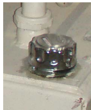
Figure 4 | Breather-filler ports and a typical replacement filter-filler.
